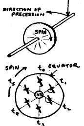
Again, if the spin axis of the gyro is in any position but the polar, the axis will move with respect to the earth's surface. This is the starting point of a gyro-compass know now that the gyro spin axis does not move with respect to the earth, when it is lined up with the North-South axis. What can we do with this?
