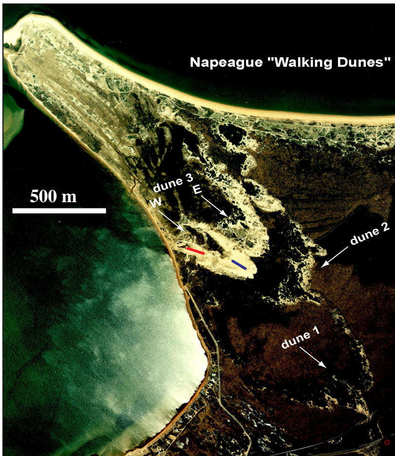
Figure 4: Aerial Image of Walking Dunes. Our primary GPR lines are from separate parts of the dune 3W. The radargram in fig. 8, indicated by the red line on this aerial image, was collected on a younger, 'small dune' forming on the western limb of dune 3W. The data from the 'big dune' (fig. 9) were collected within the main part of dune 3w (blue line). Note that the older dunes (1 and 2) are stabilized by vegetation.
