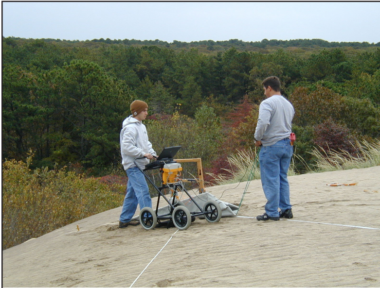
Figure 2: 200 MHz GPR survey being conducted on Dune 3w, Walking Dunes, Napeague, NY. Note that the sand is encroaching upon forest, with the tops of trees soon to be overrun by the dune.
