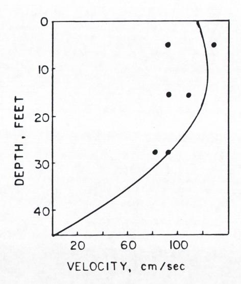
Figure 5. Profile of the distribution of the maximum tidal velocity used for the design of the buffer zone. Dots indicate measured values (Doyle and Wilson, 1979).
