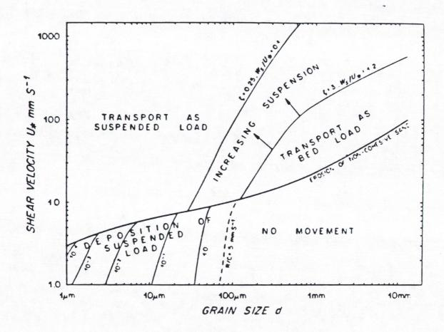
Figure 1. Critical velocities for sediment transport (McCave, 1984) including the velocities required to prevent the deposition of fine-grained sediment (less than 63 micrometers). The "shear velocity" is a measurement of the stress on the bottom; it is approximately equal to 0.0547 times the flow velocity measured one meter above the bottom (Sternberg, 1972).
