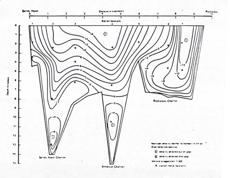
Figure 7. Average non-tidal velocities between Sandy Hook and Rockaway showing the inflow into Ambrose Channel (June 1952 from Bowman, 1977).
