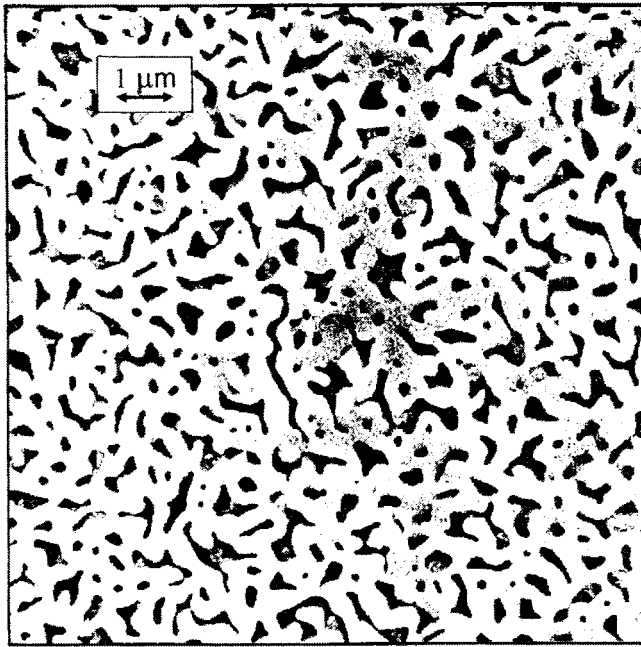
FIG. 1. Part of an electron photomicrograph of an YBCO superconducting film. The a and b axes lie in the plane of the figure, and the c axis is perpendicular to the latter.
