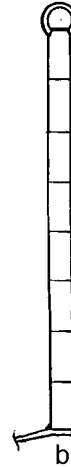
FIG. 1. Model sample of a conducting polymer composite with a grid drawn on it, as well as holes (a) and probe electrodes (b).
