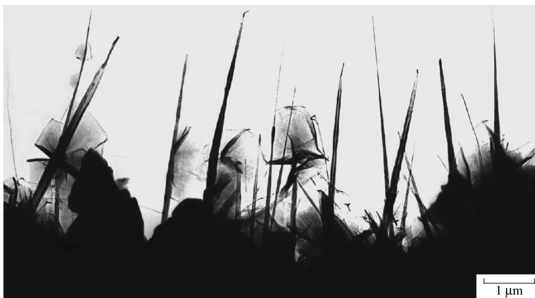
Fig. 4. A TEM micrograph of the surface of a graphite-like carbon CVD film.
