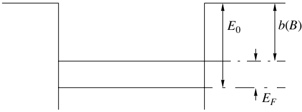
Fig. 7. The work function b(B) is the work required to extract an electron from the Fermi level of the metal. The Fermi energy E_F is measured from the minimum energy E_0 of an electron in the crystal.
