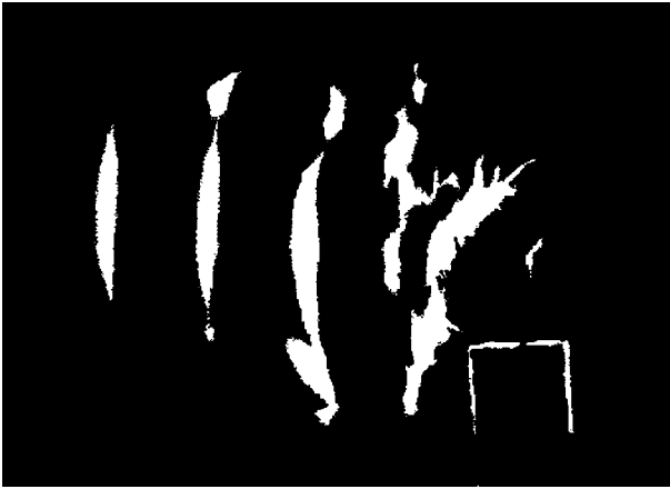
Fig. 1. An integral photograph of a “snake” structure [4]. Air, P = 100 Torr, (E/N)_0 = 100 Td, \lambda = 4.3 cm. The microwave radiation propagates from left to right.
