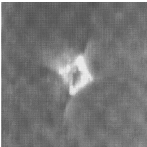
Fig. 2. A scanning photodeflection microscopy image (normal component amplitude) of the same surface region of \text{Al}_2\text{O}_3 -SiC-TiC ceramics as in Fig. 1 (the exciting laser radiation modulated at a frequency of 1.4 kHz).
