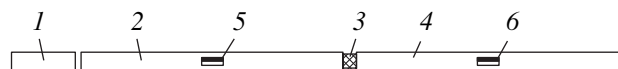
Fig. 1. Schematic diagram of the split Hopkinson pressure bar configuration: (1) striker; (2) incidence bar; (3) sample; (4) transmitter bar; (5, 6) stress sensors.
