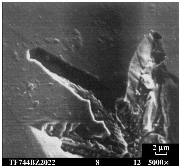
Fig. 1. Electron micrograph showing the typical shape of twins formed in a bismuth crystal loaded in a magnetic field ( B = 0.2 T; indentation time, 5 min; magnification, \times 5000 ).
