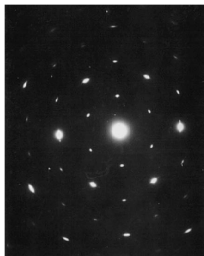
Fig. 4. Spot-type electron diffraction pattern from the mosaic CdTe film on the mica substrate.
