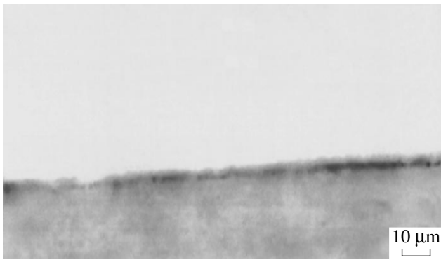
Fig. 3. An optical micrograph of the edge of a silicon sample treated with hydrogen ions for 15 min (magnification, \times 500 ).
