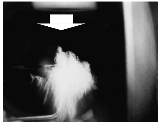
Fig. 5. The general view of a freely localized microwave discharge produced in a supersonic air flow ( M = 2 ) at a pressure of p = 350 torr, pulse duration \tau = 300\ \mu\text{s} , and repetition rate of f = 10 Hz. The microwave beam propagates from left to right. The arrow shows the direction of the supersonic flow. The arrow width is equal to the exit diameter of the Laval nozzle.
