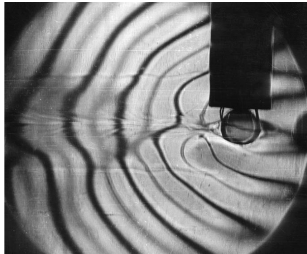
Fig. 1. Shadow pattern of a flow with isolated soaring discontinuities in the field of attached internal waves. A cylinder with the diameter D = 2.5 cm moves from the left to the right at a speed of U = 0.29 cm/s. The other parameters are T_b = 15 s, Fr = 0.28 , Re = 74 , and C = 5500 .
