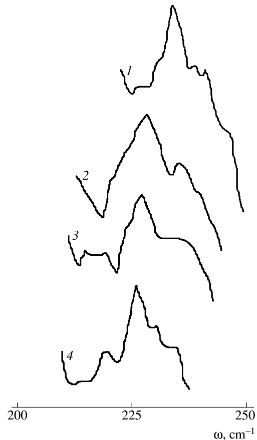
Fig. 2. Fragments of the Raman spectrum of \text{PbZrO}_3 at various strengths of the electric field near the line that has a frequency of 233 \text{ cm}^{-1} in the absence of an electric field; E = 116 \times 10^5 (1), 204 \times 10^5 (2), 226 \times 10^5 (3), 239 \times 10^5 \text{ V/m} (4); T = 293 \text{ K} .
