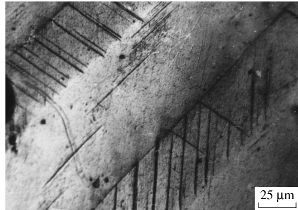
Fig. 3. Metallographic image of twinning in the case of compression of [\bar{1}11] crystals. \epsilon = 9.8\% , T_{\text{test}} = 300 K. The repeated polishing and etching were performed according to methods described in [1, 5, 6].
