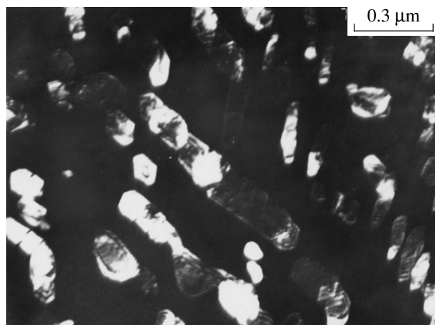
Fig. 4. Dark-field image of the perlite microstructure in the g = 1\bar{1}1_c reflection after isothermal decomposition at 600°C and additional annealing at 700°C for 30 h.
