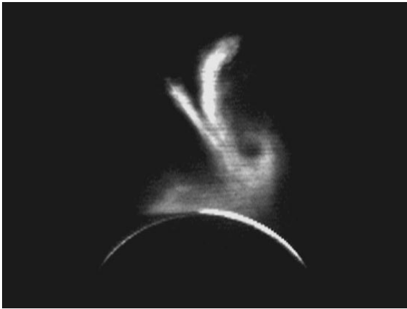
Fig. 3. Initial asymmetric pattern obtained by smoking visualization by the laser-knife method for a flow without a spark discharge for the parameters U = 15 m/s and \alpha = 17.5^\circ .
