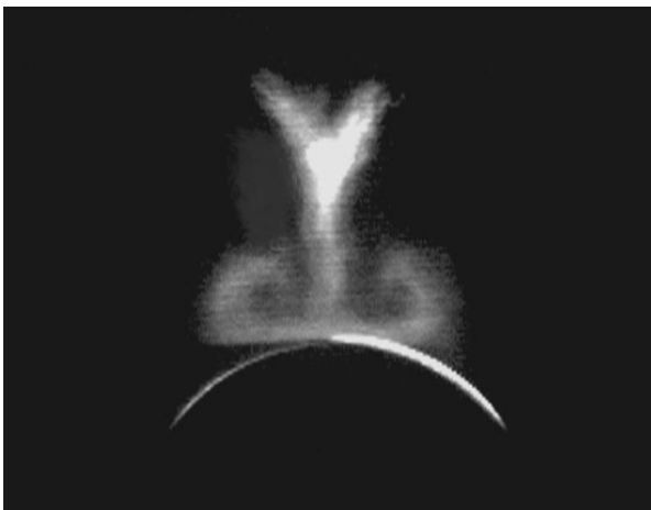
Fig. 4. Symmetric pattern obtained by smoking visualization by the laser-knife method for a flow with a spark discharge for the parameters U = 15 m/s and \alpha = 17.5^\circ .
