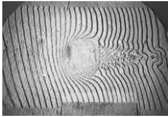
Fig. 2. Interferogram of the concentration field in the process of the bubble migration.
