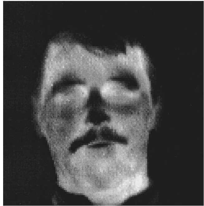
Fig. 6. The dark image obtained using a photodetector array module based on the GaAs/AlGaAs MSQWs with the size of 128 × 128. Spectral range is 7.5–8.5 μm, frame rate is 50 Hz. Operating temperature is 65 K.
