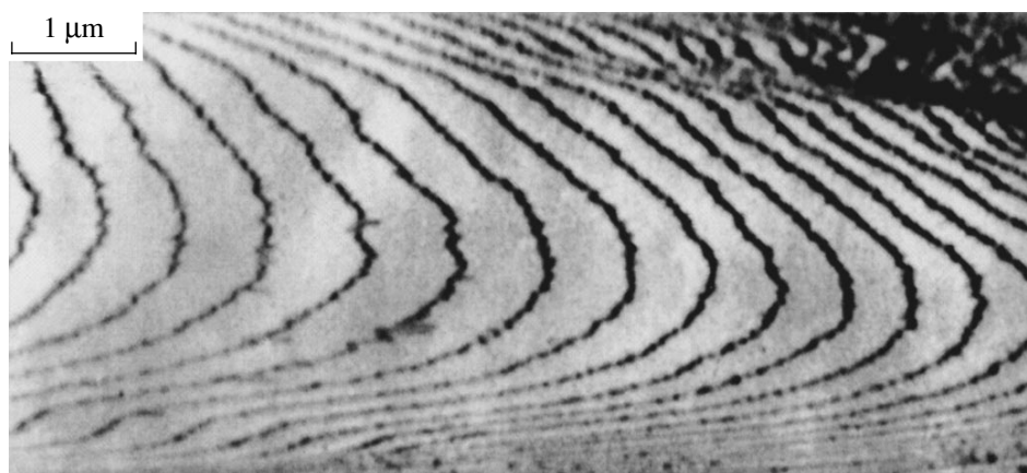
Fig. 2. Representative image of the stepped Si(111) surface exposed to the oxygen atmosphere at a pressure below P_{\text{crit}} . Monatomic steps moved from left to right.
