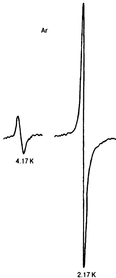
FIG. 11. EPR signals of unstable paramagnetic centers, which arise as the He gas-discharge products are trapped in a growing Ar cryocrystal. The spectrometer gains for the low- and high-temperature signals are the same. Both lines have g -factors of 1.99986(12).
