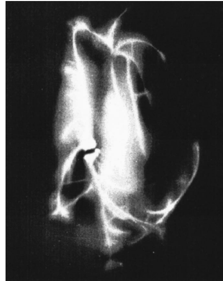
FIG. 6. Microwave discharge in helium at p=760 Torr with E_0=5.5 kV/cm.
