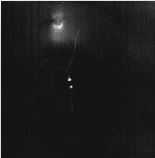
FIG. 4. Microwave discharge in hydrogen at p=300 Torr with E_0=5 kV/cm.
