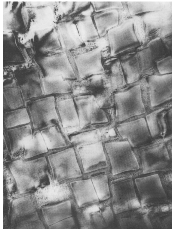
Fig. 9. Metallographic image of a two-phase A1+L 12 structure formed by cuboids of the L 12 phase with a size of about 0.2 μm in the disordered A1 phase of a Ni–Al type superalloy [22].
