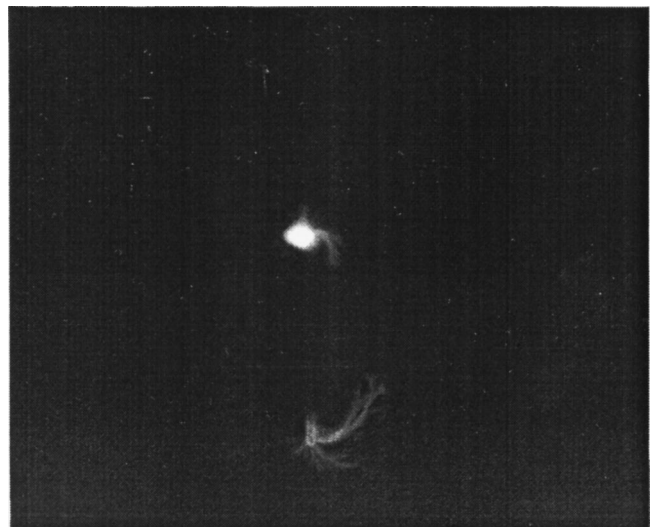
FIG. 4. A highly subcritical microwave discharge in air, which is attached to the trigger: \tau=40 \mu s , 2L=3 cm, 2a=8 \times 10^{-2} cm.
