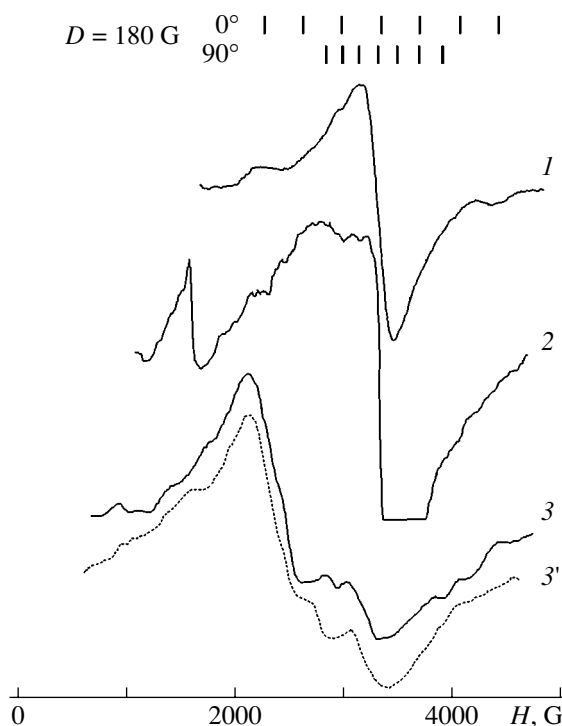
Fig. 2. EPR spectra of \text{Gd}^{3+} aqua ions adsorbed on the capillary surface: (1) 0.1 M aqueous solution of \text{Gd}(\text{NO}_3)_3 at a temperature of 298 K and the calculated position of the fine structure line at D = 180 G, (2) 0.0025 M aqueous solution of \text{Gd}(\text{NO}_3)_3 at temperatures of 298 and 100 K (in weak magnetic fields, the EPR signals are attributed to the \text{Fe}^{3+} ions involved in capillaries fabricated from conventional glass), (3) after removal of the major portion of the 0.0025 M aqueous solution of \text{Gd}(\text{NO}_3)_3 from the capillary at 298 and 100 K, and (3') the simulated spectrum at fine structure parameters D_1 = 838 G, \delta H = 250 G and D_2 = 1240 G, \delta H = 550 G. Spectra 1 and 3 are measured for samples in silica capillaries.
