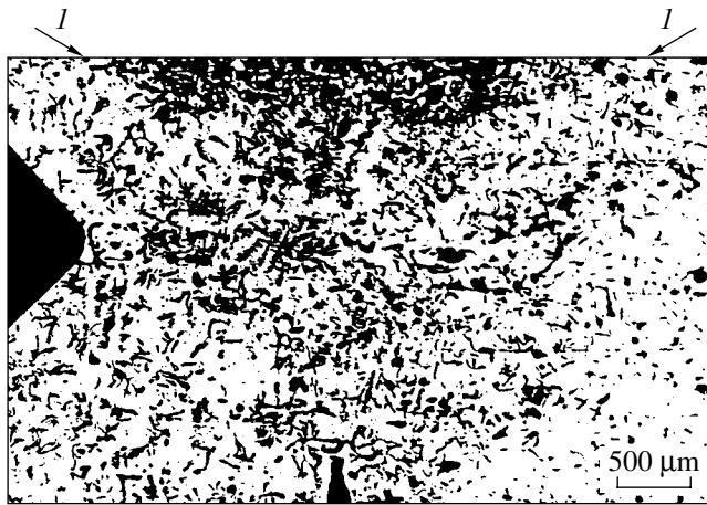
Fig. 2. Microstructure of the specular matrix zone. (I) Boundary of the molten zone.
