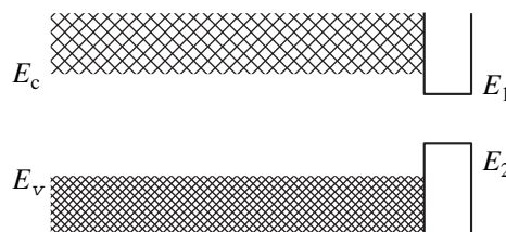
Fig. 1. Bands of ionic surface states [1]: E_c , conduction band edge; E_v , valence band edge; E_1 , acceptor surface-state band edge; and E_2 , donor surface-state band edge.
