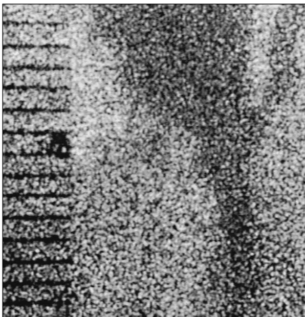
Fig. 2. Speckle photograph. Resolution 512 \times 512 pixels. The vertical scale division is 1 mm.
