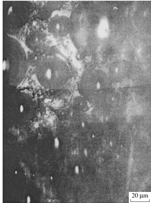
Fig. 8. Traces of plastic flow and microcracks on the fracture surface of the spheroplastic.
