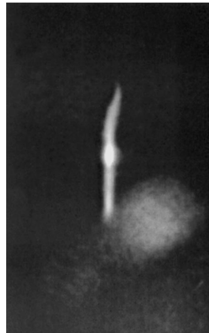
Fig. 5. Freely localized streamer microwave discharge with a high-temperature core in atmospheric air.
