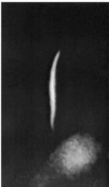
Fig. 4. Freely localized streamer microwave discharge in atmospheric air.
