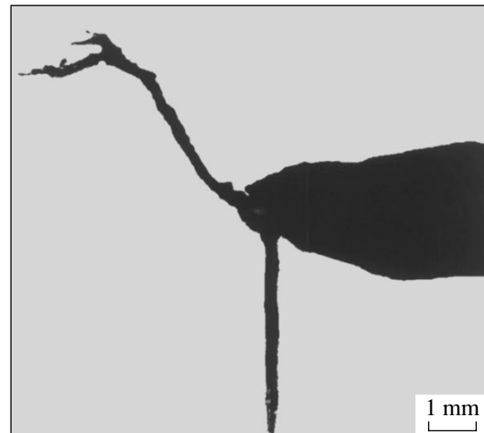
Fig. 2. Shock-wave generated secondary cracks near the edges of the initial macrocrack.
