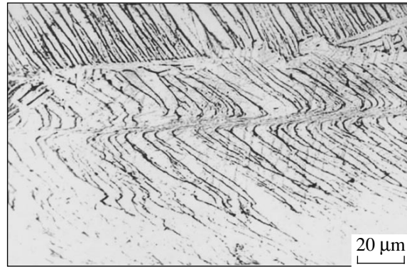
Fig. 1. Adiabatic shear band near the initial macrocrack in VT-1 alloy after dynamic loading.
