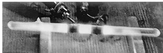
Fig. 1. RF discharge plasma glow in dry air at a pressure of about 1 kPa.
