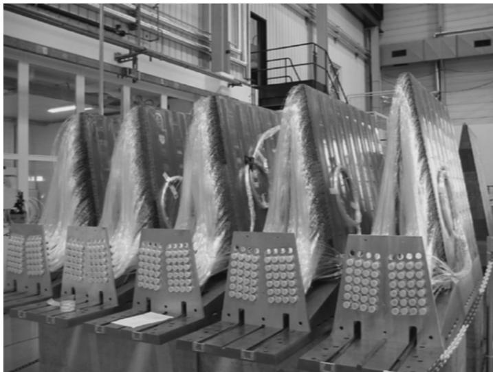
Fig. 10. Quartz-fiber-equipped sectors of the forward calorimeters of the CMS facility.
