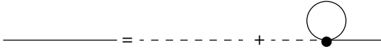
Fig. 1. The Dyson equation for the quark propagator in the Hartree approximation (solid lines). The dashed lines denote the bare quark propagator.
