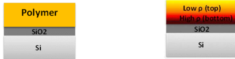
Figure 2-2 Illustration of 3-layer model (left) and 4-layer model (right) to fit the x-ray reflectivity profile.
