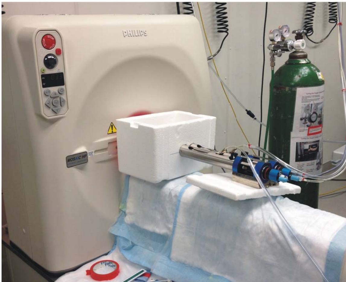
Figure 5.6 Design of PET scan with TB infected animals in BSL2 lab with BSL3 biocontainer
