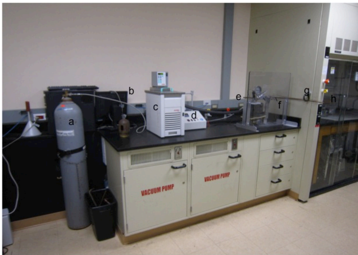
Figure 2-4. Supercritical CO 2 systems: a) CO 2 tank; b) steel tube; c) water bath; d) heat controller; e) pressure gauge and pressure vessel; f) safety shield; g) CO 2 venting tube; h) Fume hood
