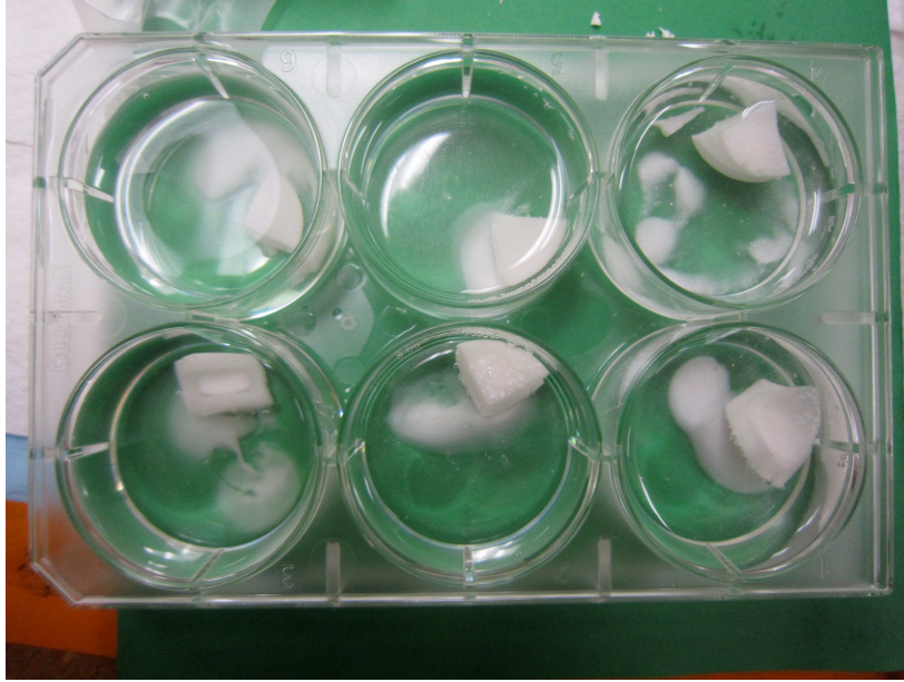
Figure 3-8 EDC/NHS cross-linked gelatin/starch/HA scaffold after 7 days of immersion in SBF at 37°C. All the samples were cross-linked by soaking in DI water containing 34 mM EDC and 17 mM NHS for 24 hours.
