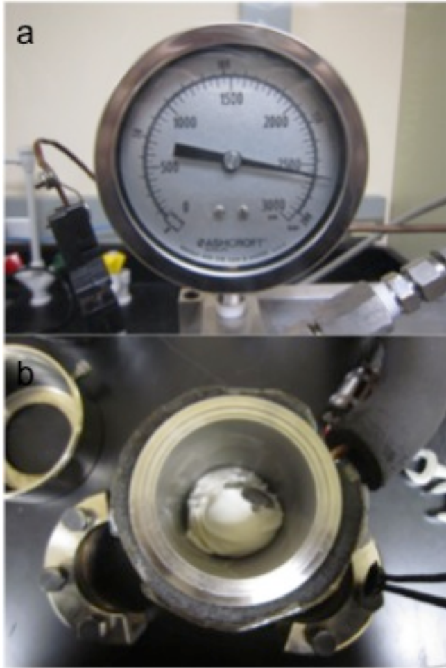
Figure 2-3. a) Pressure gauge used to monitor SCF process; b) Supercritical CO 2 high-pressure vessel
