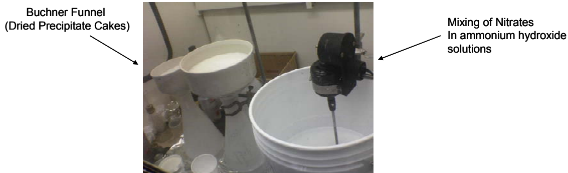
Figure 14 Batch processing was required to create over one kilogram of desired powders. Photograph depicts mixing container, chemical mixer and large filtration used to produce precipitation cakes.
