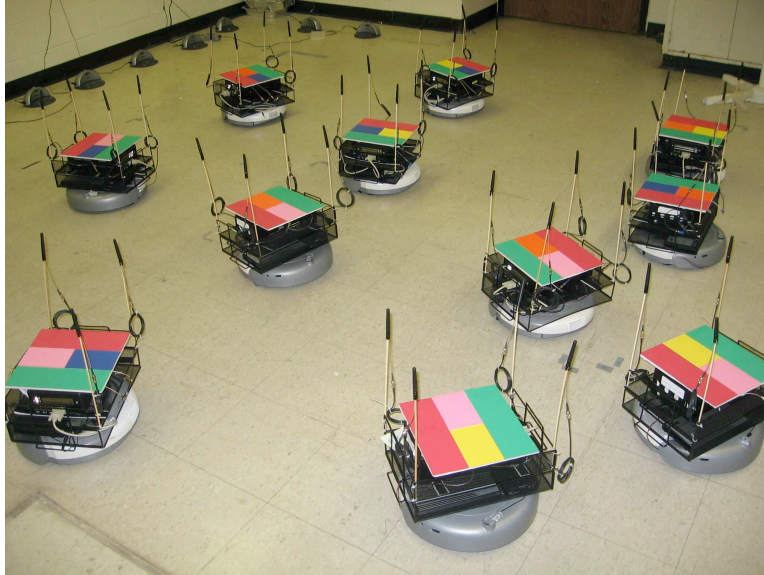
Figure 31: MiNT-m prototype with 12 mobile nodes and charging stations (top left corner of the image).
