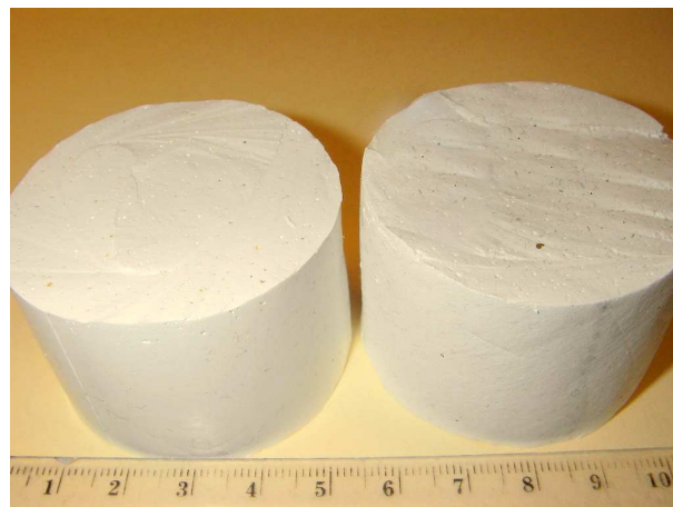
Figure 5.3: The left and right cylindrical specimens are “hard” and “soft” silicone, respectively. The dimensions of both specimens are 25 mm in radius and 30 mm in height.
