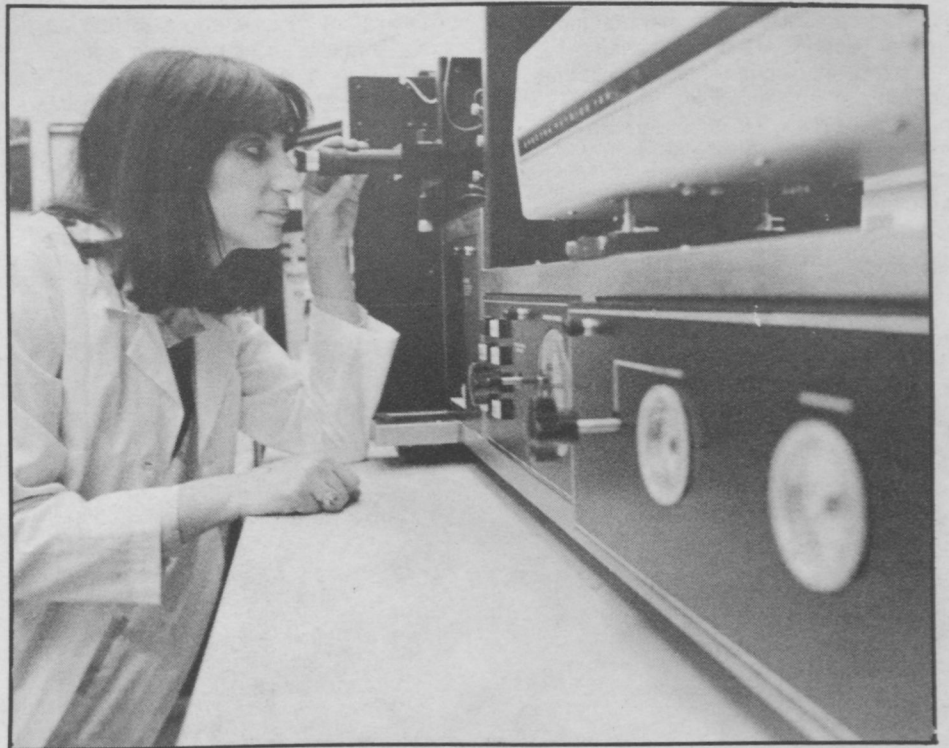
Laser analysis of white blood cells, performed by the Coulter Epics V Fluorescence Activated Cell Sorter, allows research assistant Joanne Thomas to diagnose Lyme disease.
