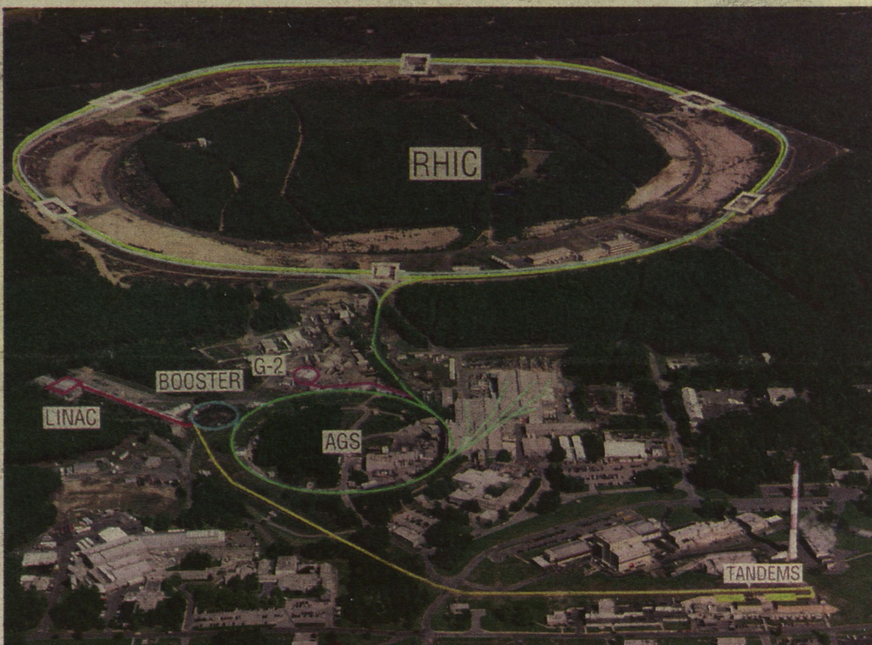
The RHIC complex, showing the path of the ion beam from the "starting line" at the Tandem Van de Graaff accelerator at bottom right, to the "warmup track" of the Alternating Gradient Synchrotron (AGS) in the center, to the 3.8-kilometer RHIC ring at top. At six points around the ring, the two beams will be brought together to collide, releasing particles for physicists to study. (Photo courtesy BNL)
