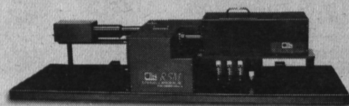
OLIS RSM CD UV/Vis dual-beam phase-coherent spectrometer
