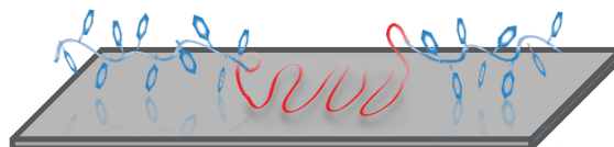
Fig. 3-5. Proposed SBS chain conformation on the substrate
