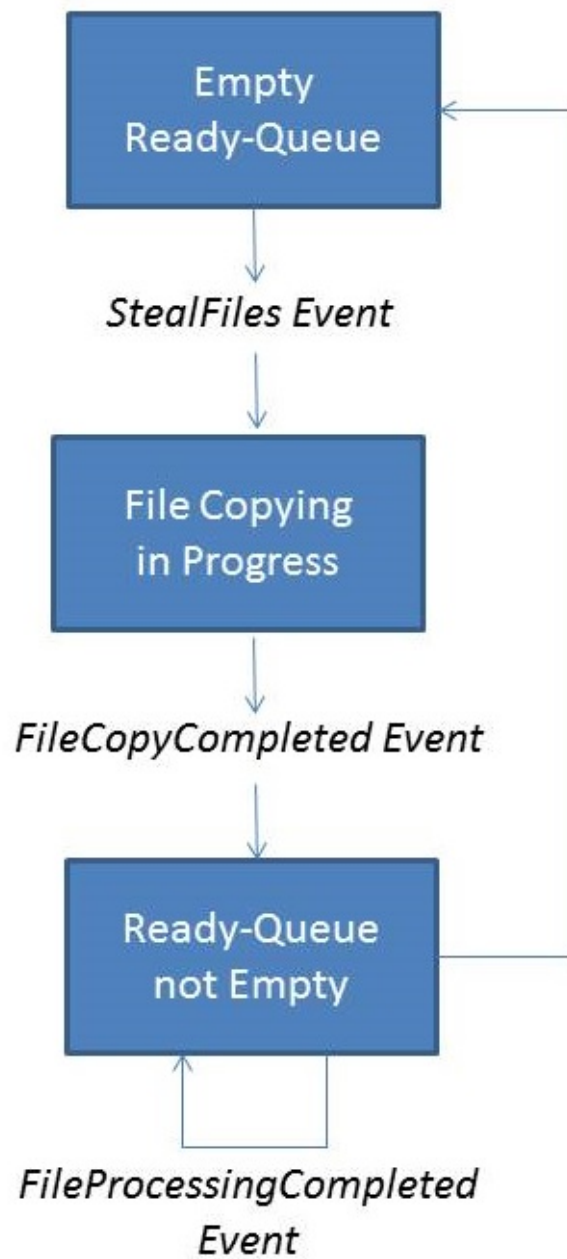
Figure 3.2: The sequence of discrete-time events that can occur on each processing machine during the e-Discovery workflow.
