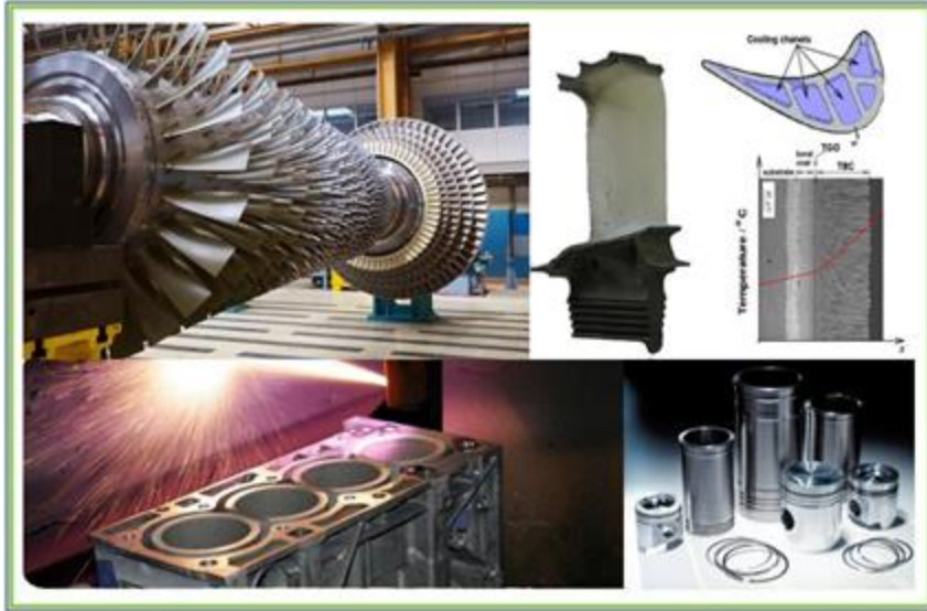
Figure 1. Illustration of TS coatings applications at medium and high temperatures (Siemens)
