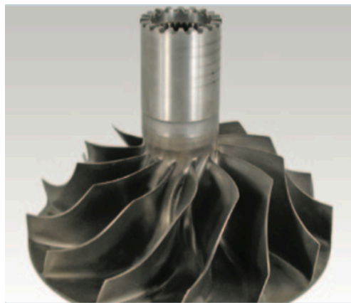
Fig. 2.5 Impeller repaired by the LENS 850-R 15
