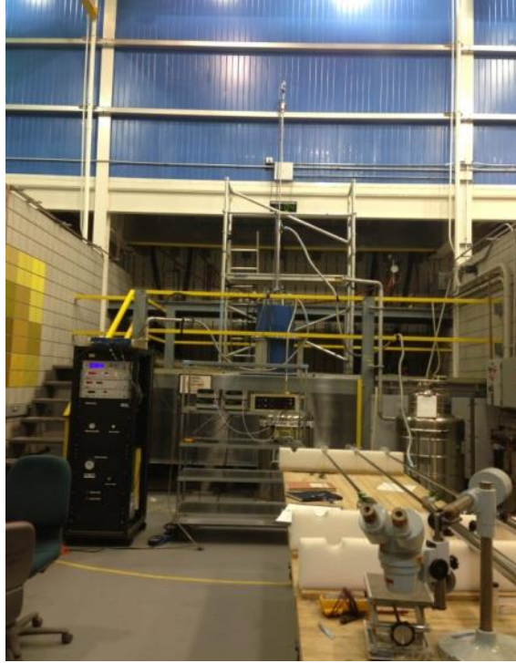
Figure 2.15 Cell 12 in National High Magnetic Field Laboratory, equipped with a 34.5 T magnet.
