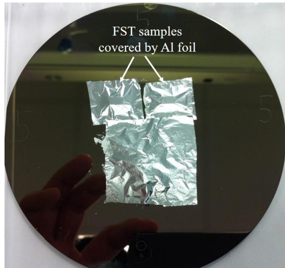
Figure 2.8 \text{FeSe}_{0.5}\text{Te}_{0.5} samples on a 4-inch silicon wafer covered by 1.5\ \mu\text{m} Al foil, prepared for being irradiated by protons.
