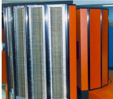
Figure 3.6: The Cray X-MP with processors stacks in circular arrangement, typical of Cray machines. It was capable of performing 800 Megaflops
