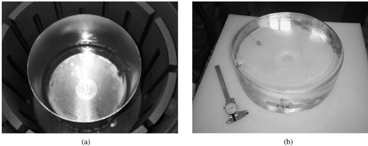
Figure 1.10 HEM sapphire boules, 34 cm diameter, 65 kg (a) after growth still in the crucible, and (b) after removal from the crucible [13].
