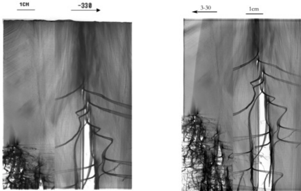
Figure 3.10 Reverse g reflections taken according to first setting in Figure 24, left one is reflection g = -3300 , right one is reflection g = 3-300
